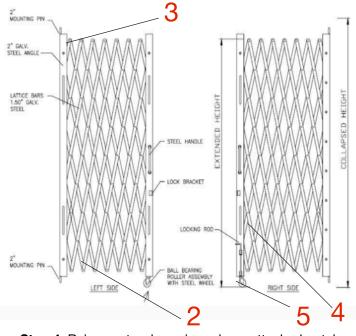
**Step 4:** Raise center drop pin and use attached notch to keep in place, this prevents damage to floor surface. Extend and retract gate to its stops to work out stiffness. Repeat steps 2-3 for other half of gate. CAUTION: Notice that center drop pin at this stage hits the other half of gate or rests on floor. Do not cut off drop pin. Step 5 addresses misalignment.
